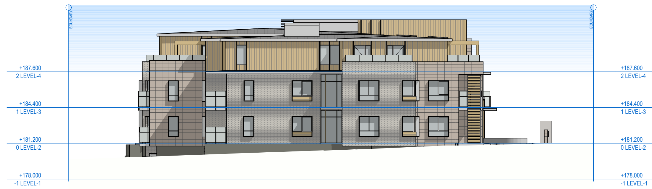
E02 SOUTH ELEVATION - COLOURED SCALE: 1:200 0 5.0M 10.0M
